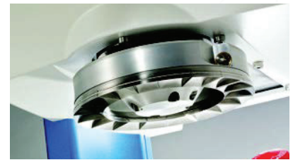
Close-up View of Vane Lid used for Flow Function Test
