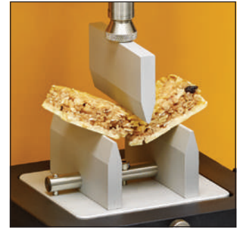
TA-TPB F Three Point Bend Fixture is used with TA7 blade from general probe kit. Fixture Base Table required. Small scale version TA-JTPB is available.
