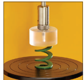
TA11 D Cylindrical probe TA11 is used to measure the force vs. distance in mechanical springs. TA11: included in TA-P-KIT2 or as a standalone part.
