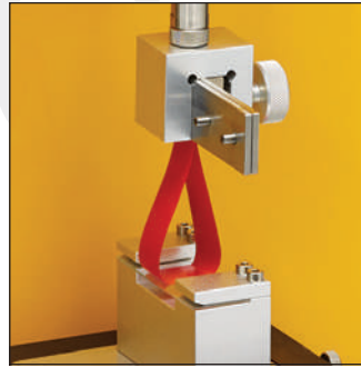
TA-LTT M Loop Tack Test measures the adhesive strength of pressure sensitive tape and stickers according to ASTM D6195.
