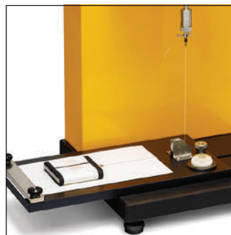
TA-SFJ M D Sliding Friction Jig measures the coefficient of friction for packaging materials according to ASTM D1894.
